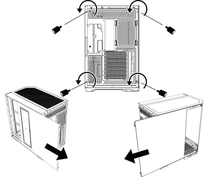
How to remove the dust filters/Comment retirer les filtres anti-poussière
